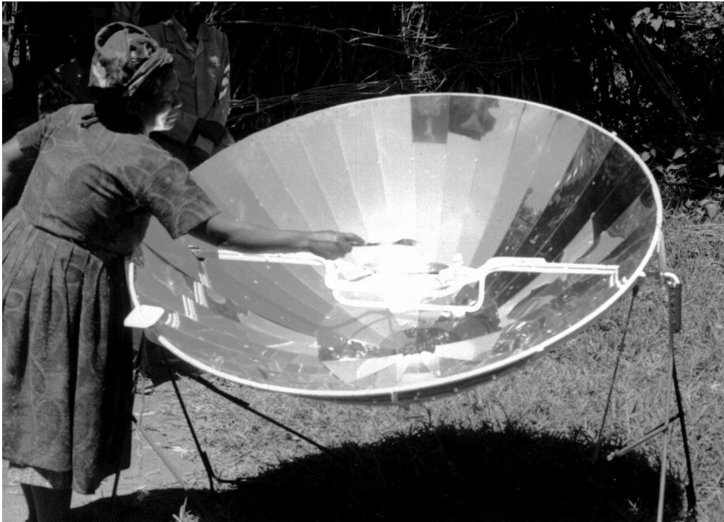
Figure 1: Roasting coffe with the AMSI solar cooker
